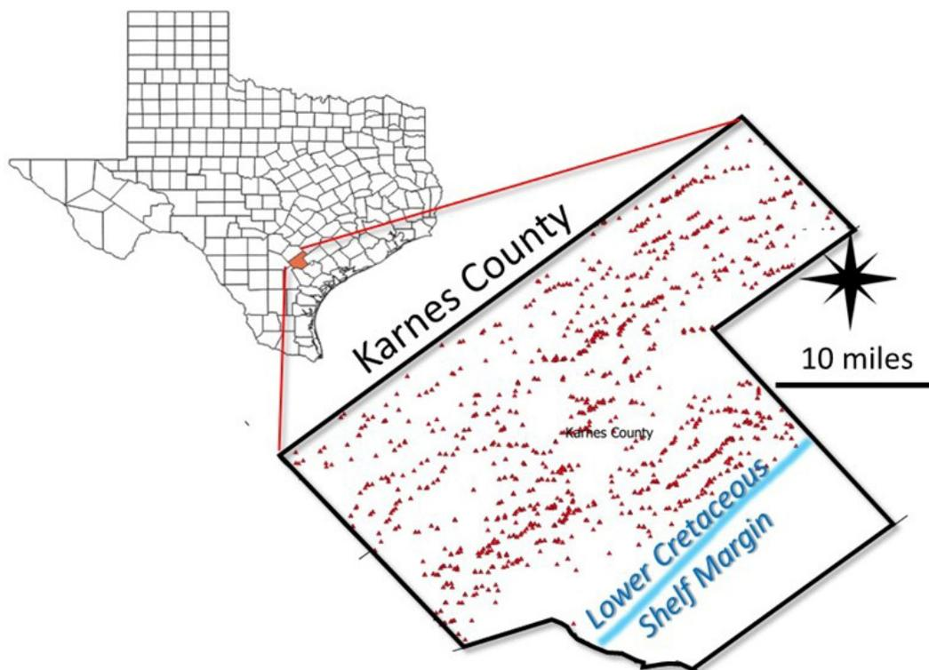
Figure 1. Location of the Karnes County study area in South Texas. Red dots show well-head locations for Eagle Ford wells used in this study. Drilling is confined to areas up dip (i.e., to the northwest) of the Lower Cretaceous shelf margin that underlies the Eagle Ford.
