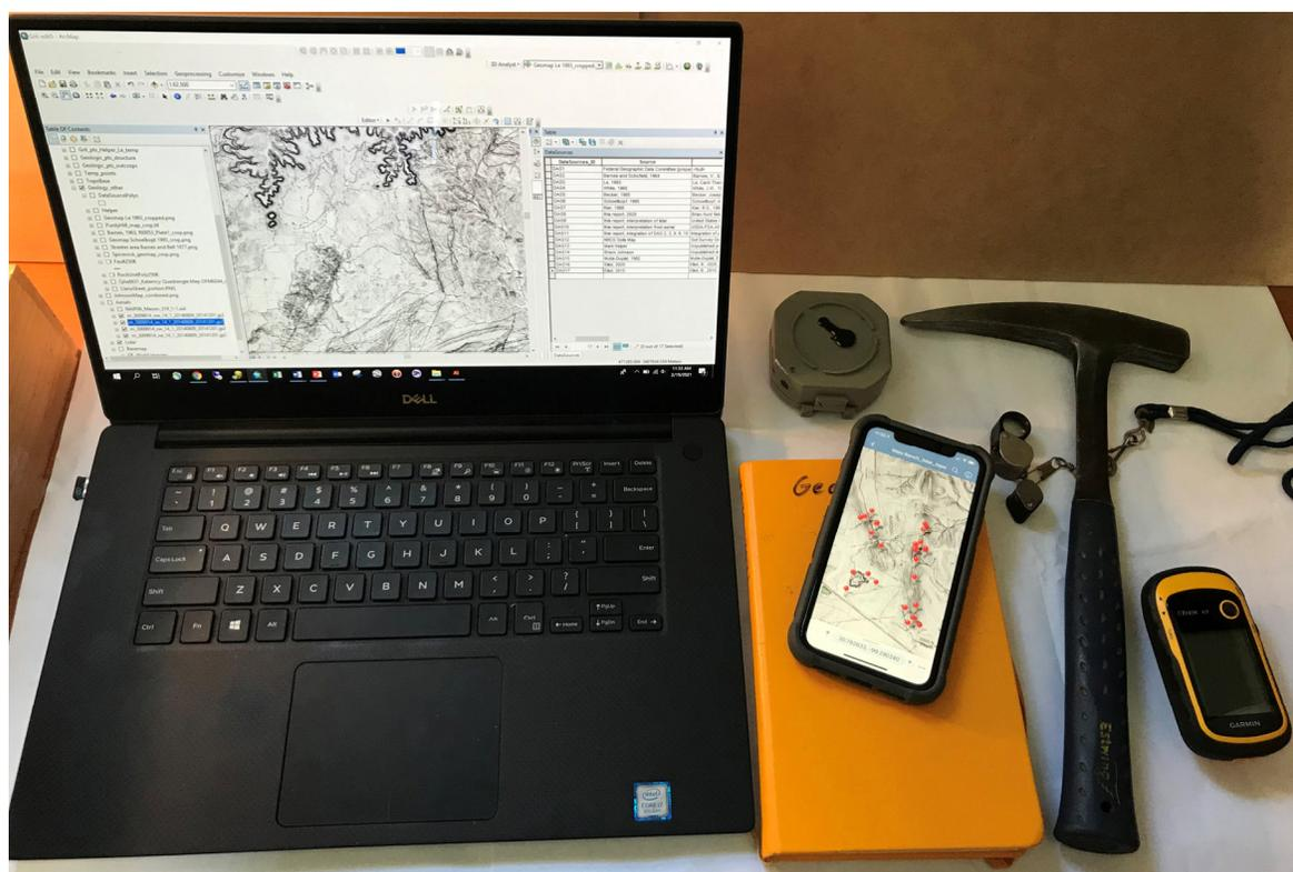
Figure 1. Photograph of mapping tools used in this study (from left to right): laptop with GIS, iPhone with mapping application, Brunton compass, field book, hand lens, hammer, and backup GPS.
