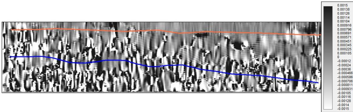
Figure 7. Curvature in dip direction using 15 Hz trace decomposition as input. As in [Figure 2](#), the dipping strata continue to be enhanced throughout the lower Vicksburg and are almost absent below the glide plane.
