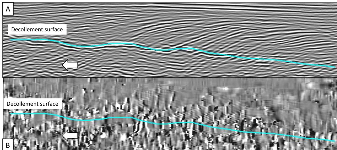
Figure 2. Cross-section showing seismic profile across the foreset sequence. Orange line defines the top of the sequence. Blue horizon indicates the decollement in Jackson Formation (Eocene) shale. (A) Reflection profile showing strong imbricate foreset beds in the right-hand half. (B) Curvature (in dip direction) attribute, based on reflections, displaying high-resolution coherent events related to reflections.
