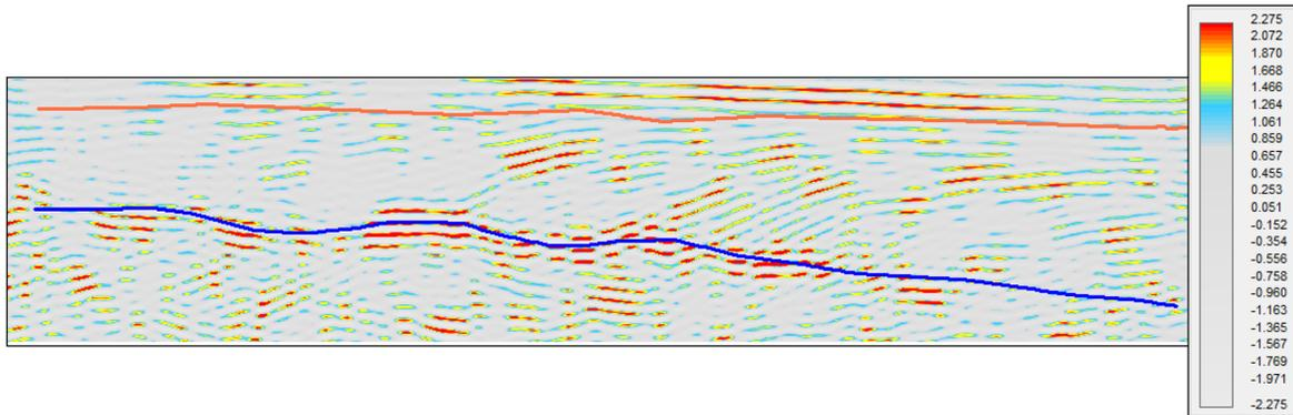
Figure 6. Spectral decomposition, trace calculation, 15Hz center band. Onlaps, toplaps, downlaps, and Vicksburg fault zone are clearly preserved and enhanced with respect to [Figure 5](#).
