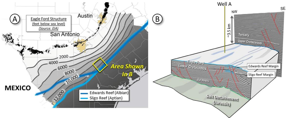
Figure 1. (A) Location map showing simplified structural contours on top of the Eagle Ford. Yellow box shows approximate location of dataset used in this study. (B) Annotated seismic imagery showing broad-scale structural configuration, ages of main stratigraphic units, and approximate location of the well used in this paper. This paper focuses on the Upper Cretaceous and Tertiary section above the Eagle Ford.
