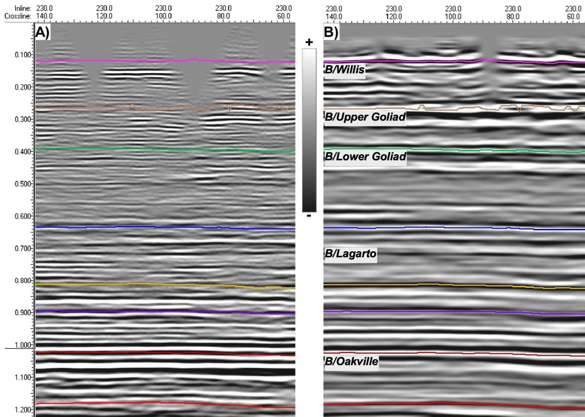
Figure 8. Comparison of original processing vs. 2021 reprocessing; note great improvements above 600 msec to about 100 msec (two-way travel time).
