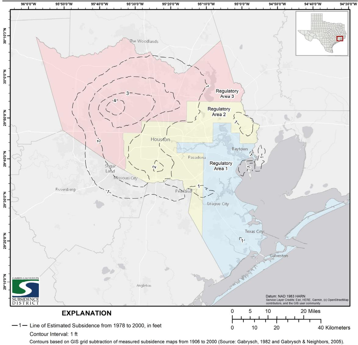
Figure 6. Total estimated subsidence from 1978 to 2000, in feet, utilizing GIS grid subtraction of measured subsidence from 1906 to 1978 (Gabrysch, 1982) and measured subsidence from 1906 to 2000 (Gabrysch and Neighbors, 2005).
