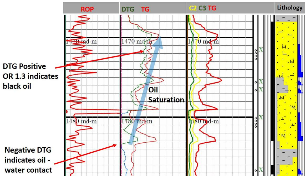
Figure 6. Oil-bearing interval with a downward oil-saturation decrease trend until it reaches the oil-water contact, where DTG becomes negative within the free-water filled zone. TG still shows elevated values and GC shows heavy gas components are slightly increased not indicating the oil-water contact position.
