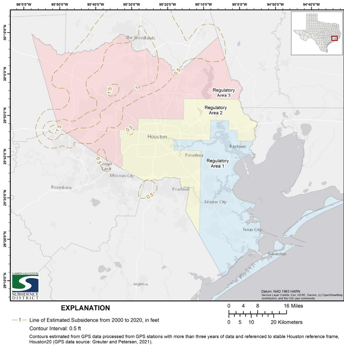
Figure 7. Total estimated subsidence from 2000 to 2020, in feet, estimated from GPS data acquired from approximately 225 GPS stations, located within the subsidence monitoring network, with more than three years of data.
