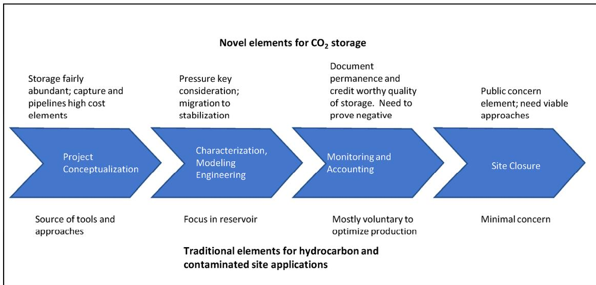
Figure 2. Components of a CO<sub>2</sub> storage project showing novel (top row) and well-established (bottom row) elements.
