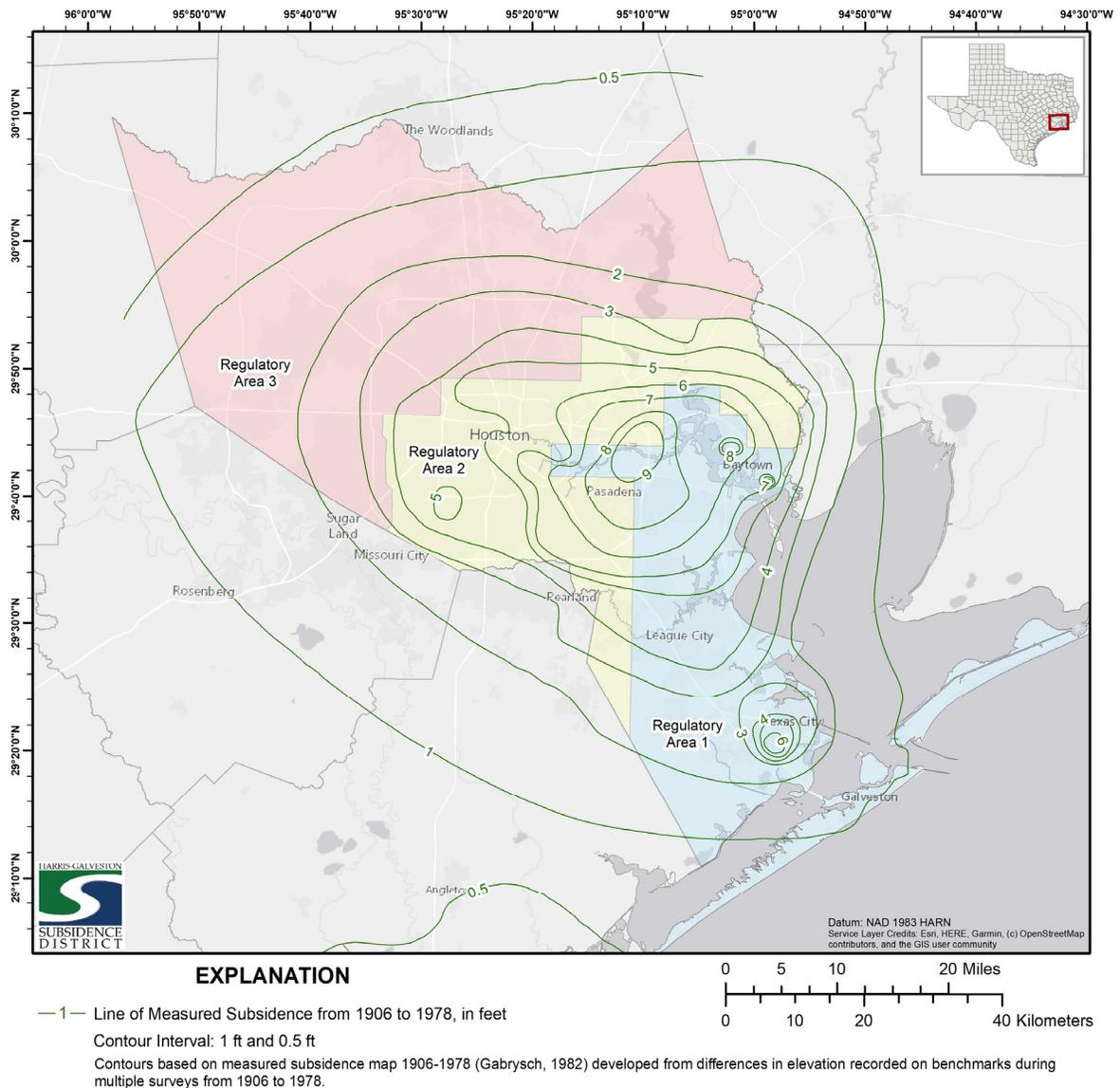
Figure 3. Total subsidence from 1906 to 1978, in feet, measured from differences in elevations at benchmarks surveyed from 1906 to 1978 (modified after Gabrysch, 1982).
