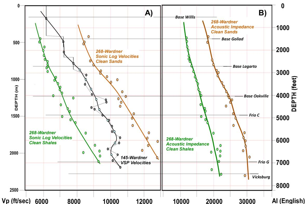
Figure 6. (A) Velocity vs. depth and (B) acoustic impedance vs. depth for clean Gulf Coast sands and shales in the Stratton area, Nueces County, Texas. Sandstones are faster and higher impedance than shales, with difference remaining fairly constant with depth.
