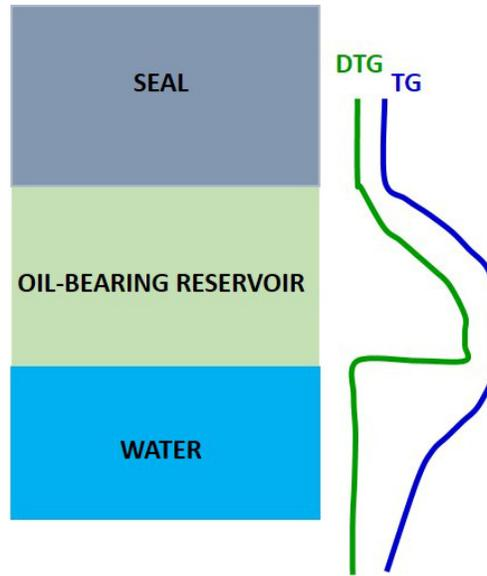
Figure 1. Oil-water contact is indicated by the sharp drop of the DTG curve whereas the TG curve has a bell-shaped anomaly.
