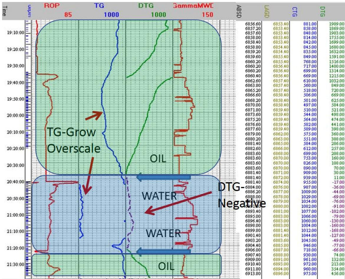
Figure 3. TG and DTG curves observed during the horizontal drilling through Austin Chalk. TG indicates gas show throughout the interval. However, the DTG curve is decreasing and becomes negative within the 6880 to 6905 ft interval, indicating that the well is penetrating a water-saturated interval interpreted to be associated with the fault. Notice that TG is increasing within the water-saturated zone due to the high concentration of methane in it.
