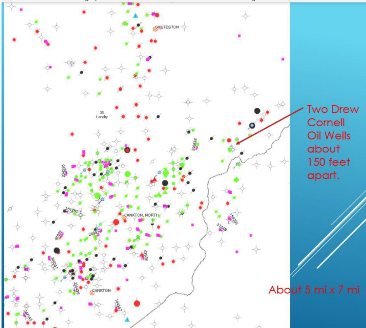
Figure 5. Well spots in the area of Cankton and Shuteston fields in southern St. Landry Parish, Louisiana. This is an example of fields which were developed with little to no seismic data...certainly no 3D data. These fields have reservoirs from a couple of thousand feet to really deep...perhaps >20,000 ft. The shallow reservoirs are certainly under-drilled. The arrow indicates the two Drew Cornell and Associates wells discussed in the text.
