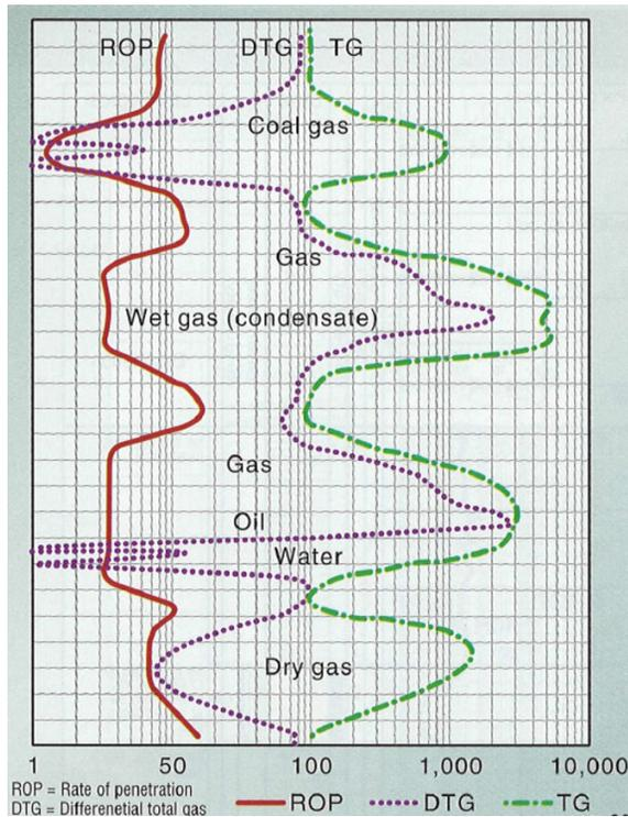
Figure 2. Differential Total Gas (DTG) and Total Gas (TG) curves interpretation chart and oil ratios differentiating fluid types within the reservoir.
