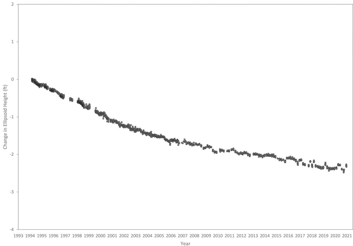
**Figure 5.** Period of record GPS–derived time series plot for GPS station P001, located in Jersey Village, Texas. The vertical displacement, as shown in the change in ellipsoidal height, from 2000 through 2020 was used to estimate the subsidence experienced at P001. This value was used as input to model the estimated subsidence contours from 2000 to 2020.
