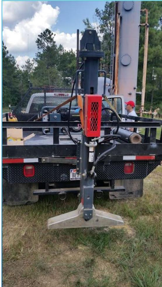
Figure 1. A-200 nitrogen accelerated weight-drop seismic source. Photo credit: Nathan Quick.
