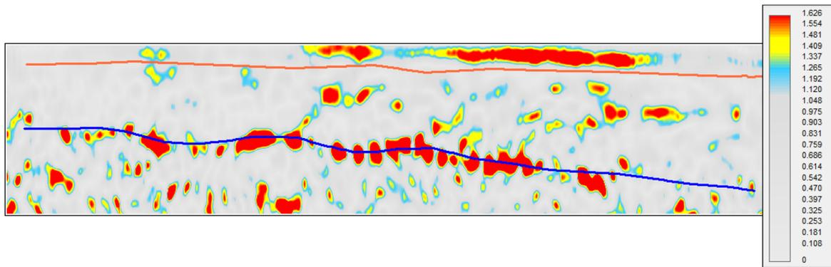
Figure 5. Example of spectral decomposition, trace envelope option, center frequency is 18 Hz. The Vicksburg Fault Zone is well defined, but onlap and toplap packages do not stand out from the background. Top (orange) and base (blue) of lower Vicksburg are included for reference.
