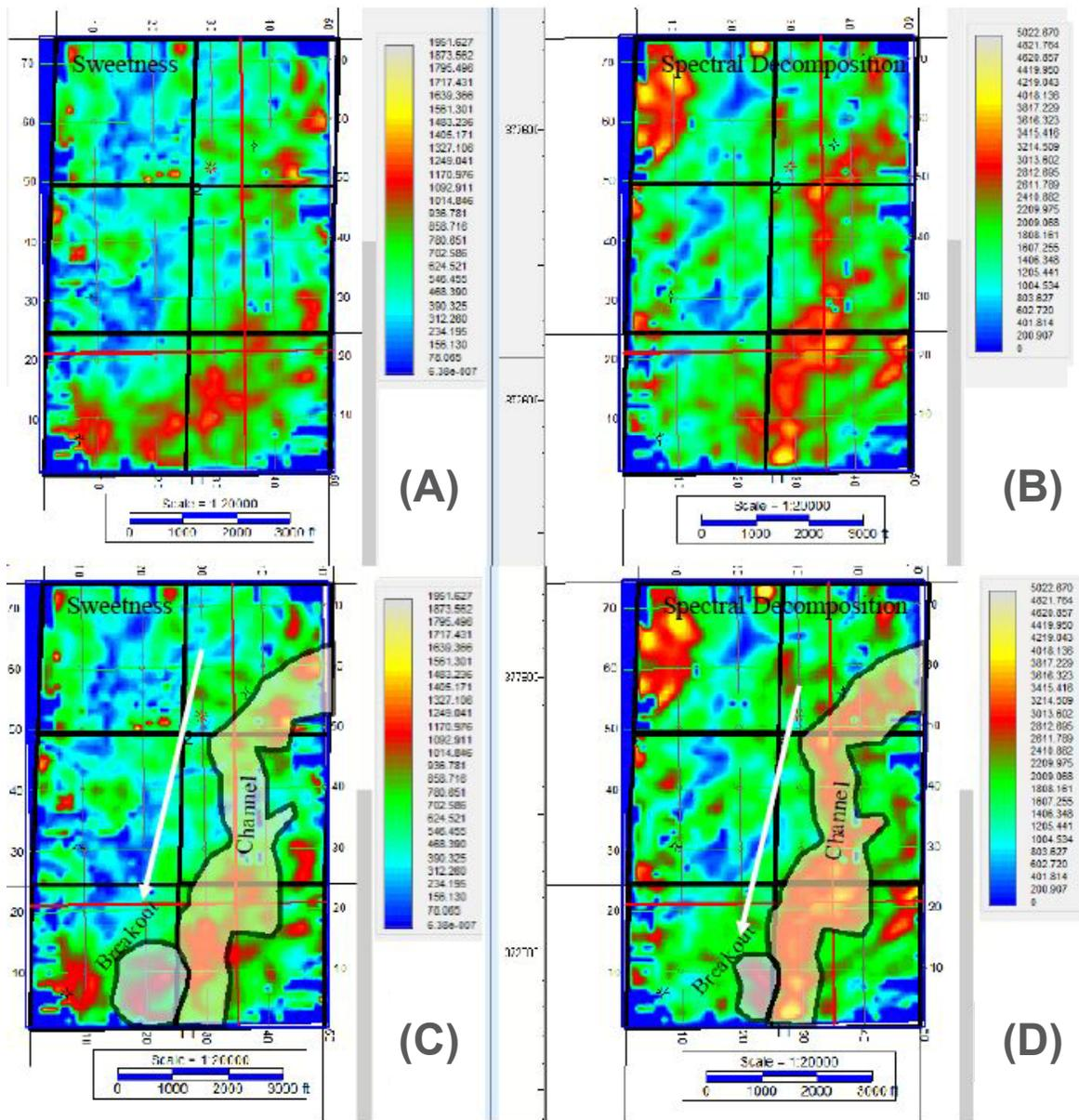
Figure 4. Small 3D from Grant Parish collected with the SSSD technique. Uninterpreted and interpreted stratal slice illustrating the ability of the data to image a small channel (modified after Stelly, 2019). Squares are 1/2 mile squares...not sections. The channel deposit is imaged even where it is less than a few hundred feet across. North is to top.
