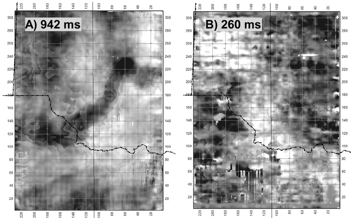
Figure 10. Geologic channel features in the Miocene imaged on the reprocessed data; time slices are flattened on nearby high-quality reflectors. (A) Channel in the Upper Oakville (942 msec, 3260 ft); (B) channel in the Upper Goliad (260 msec, 800 ft), which appears to be the shallowest geologic feature imaged.
