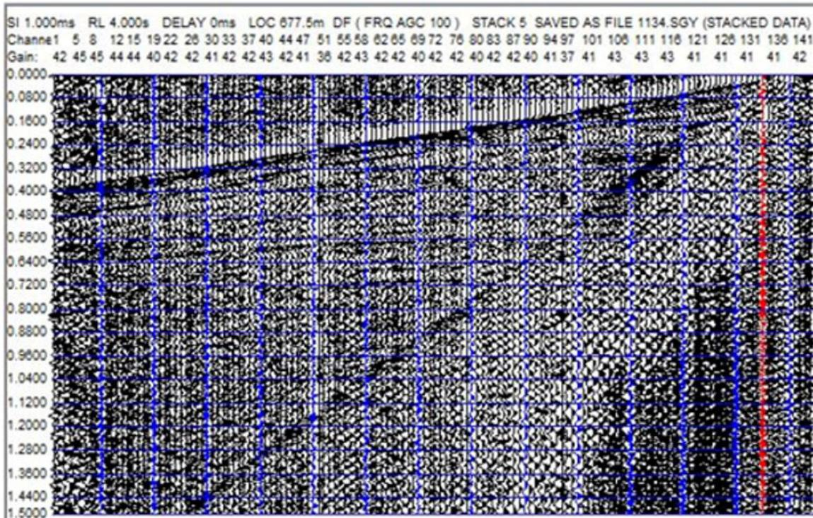
Figure 2. Screen image of a shot gather as recorded in the field. Our “minimum” target, the Carrizo Sand, is clearly imaged as a hyperbolic reflector with a far offset (left edge) time approximately 0.6400 sec. Several other reflectors are evident both above and below the Carrizo in this single fold (5 impacts stacked at one source point) record.
