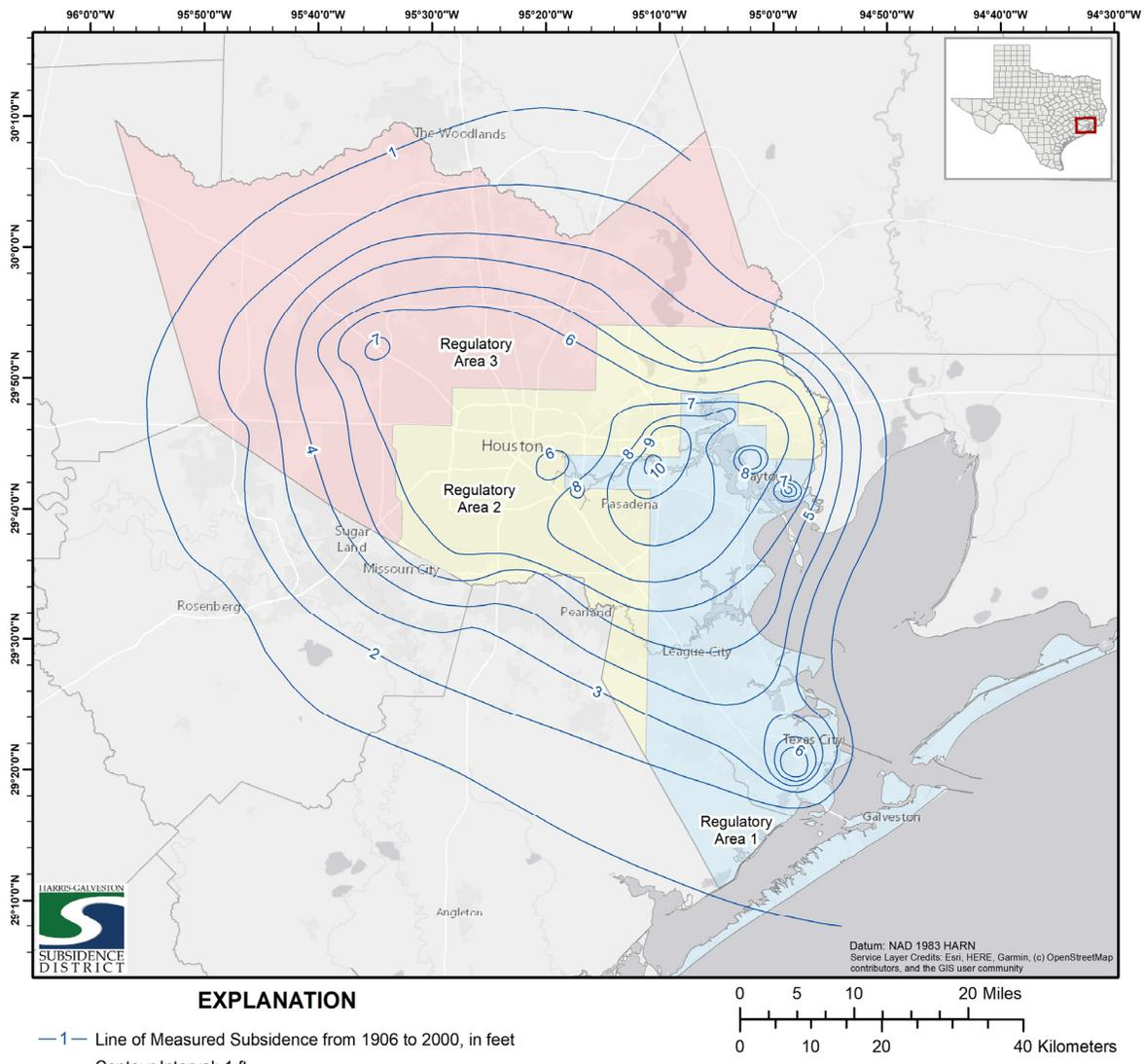
Figure 4. Total subsidence from 1906 to 2000, in feet, measured from differences in elevations at benchmarks surveyed from 1906 to 2000 (modified after Gabrysch and Neighbors, 2005).
