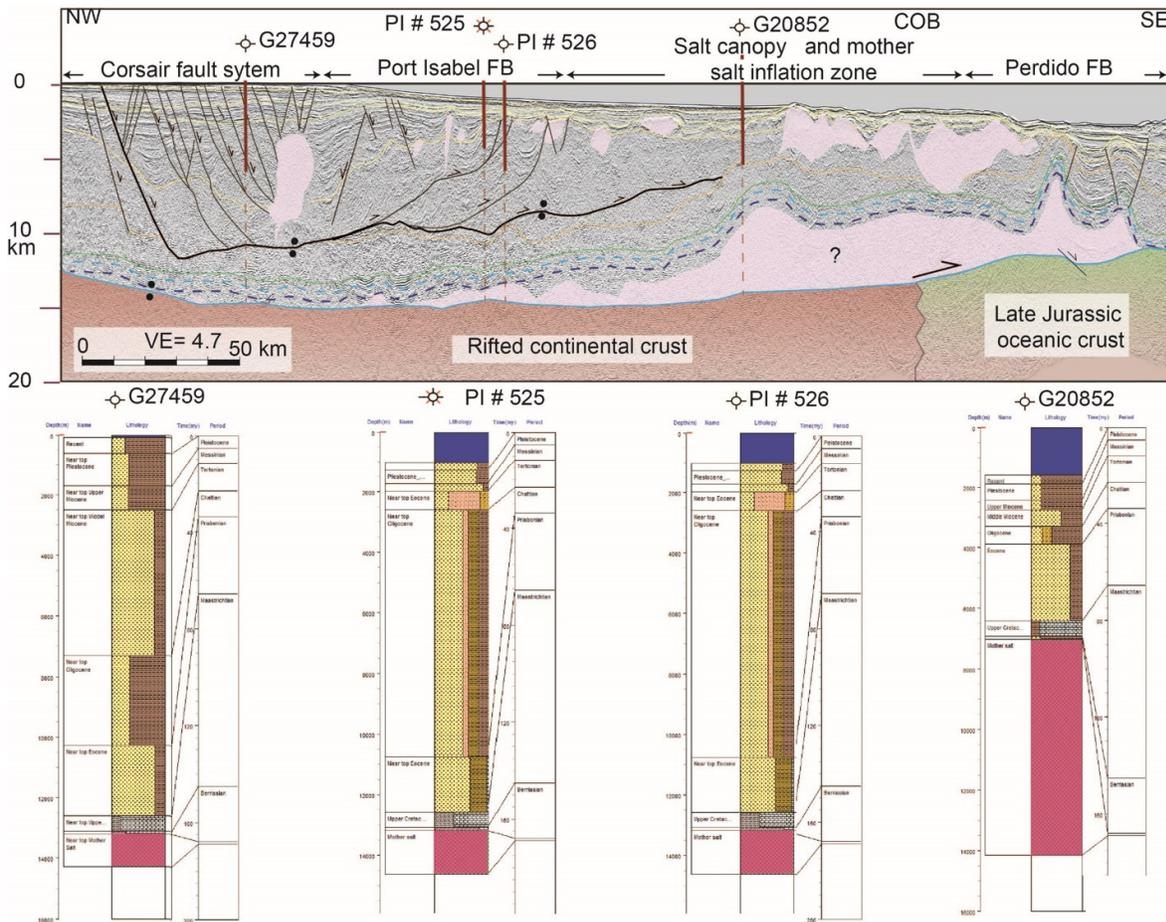
Figure 3. Interpreted dip regional seismic section showing the mapped seismic horizons in the study area. Existing drilled well locations and their simplified lithology are highlighted. The lithologies are compiled from Fiduk et al. (1999).
