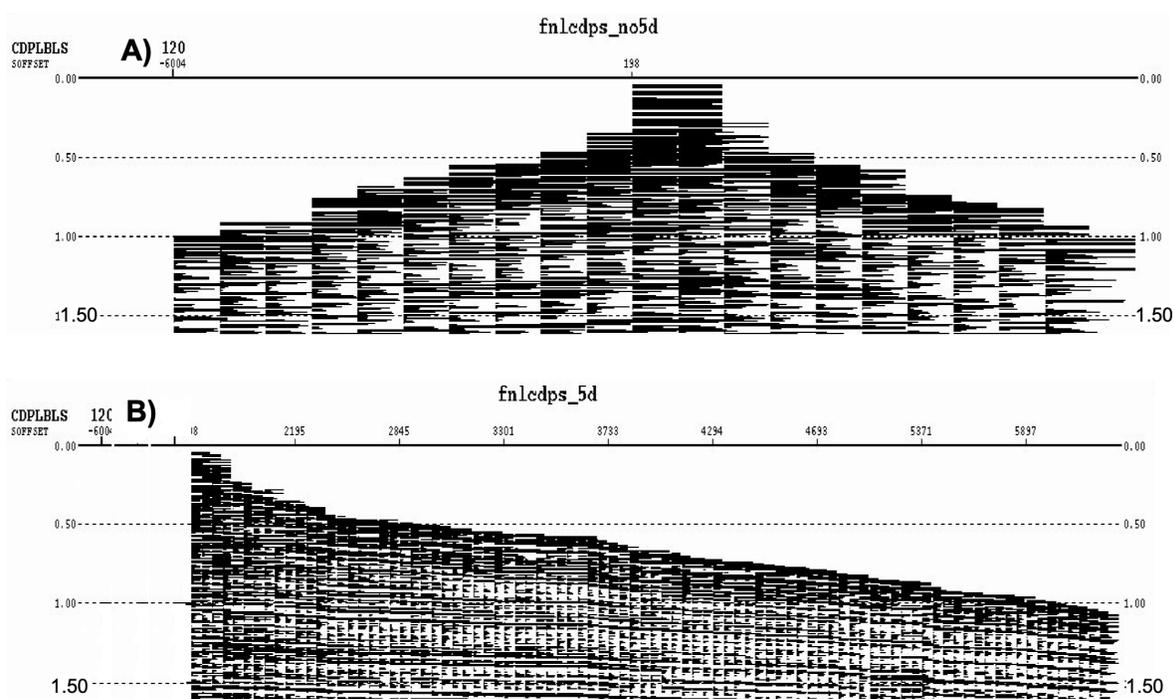
Figure 9. Typical bin gather (A) after rebinning to square bins but before interpolation; and (B) after interpolation (only half the spread shown), showing increase in data and increased ability to determine velocities.
