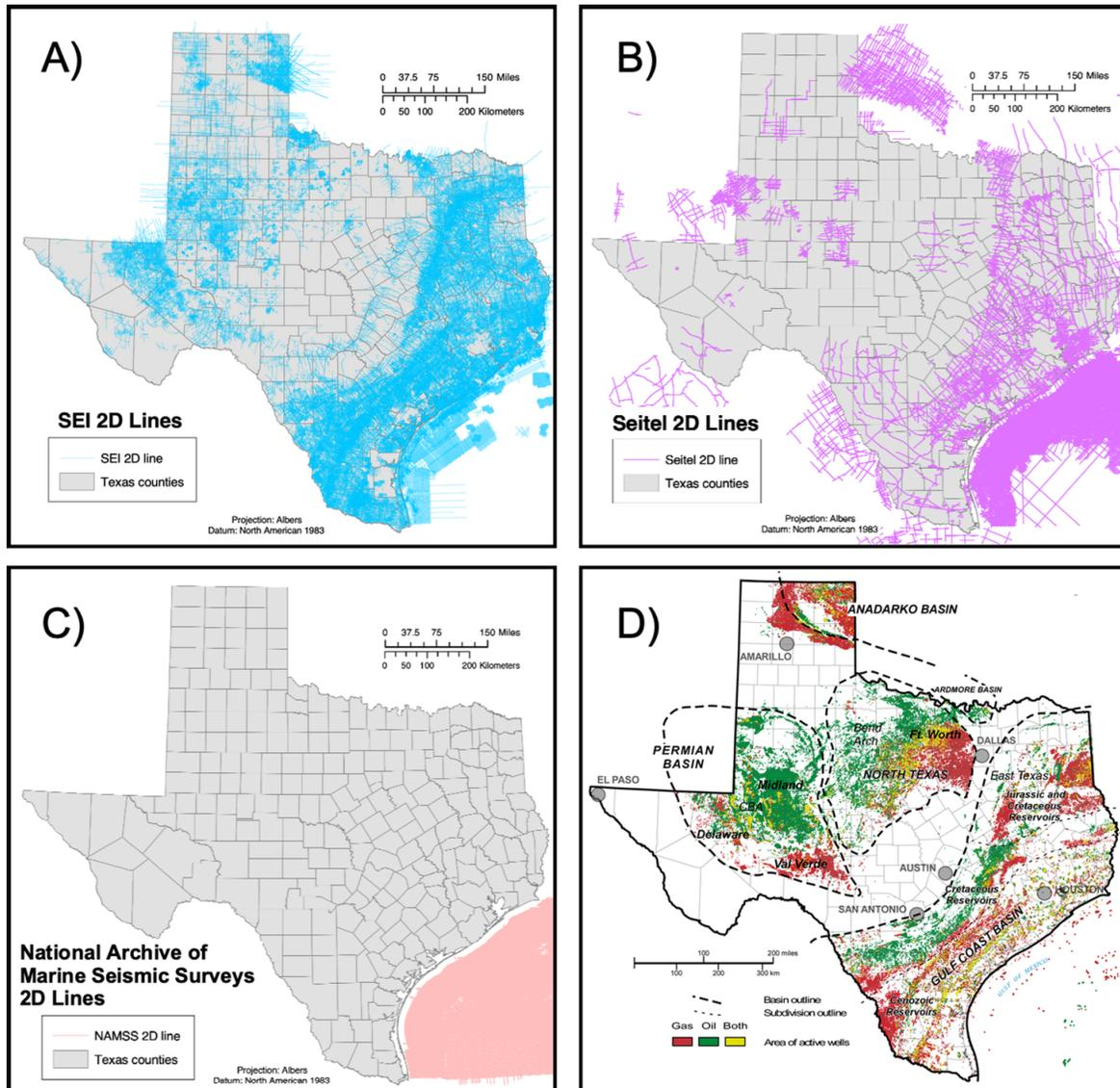
Figure 2. Availability of 2D seismic profiles in Texas and the Federal OCS, by vendors. Map of oil and gas fields and basins is from Ewing (2016). Significant amounts of 2D data are still held proprietary and are not shown.
