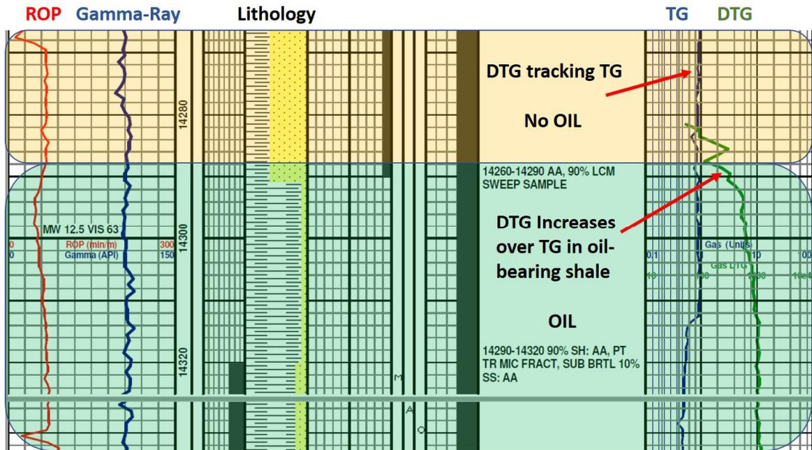
Figure 7. DTG and TG curves behave identically within the sand part of the well. However, within the shale oil interval DTG clearly increases while TG curve does not go up and at places TG readings even decrease.
