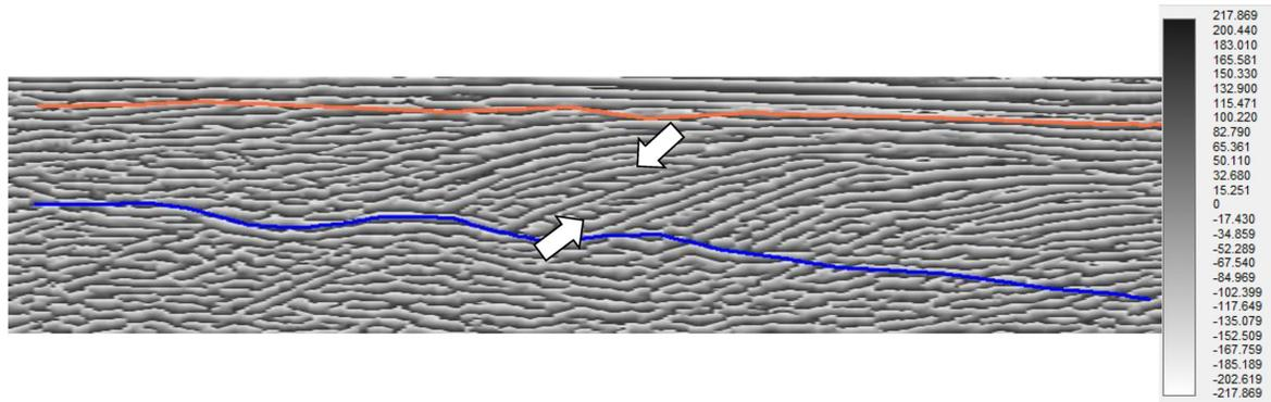
Figure 8. Instantaneous phase extraction from data displayed in [Figure 7](#). Depositional features in the lower Vicksburg sediments are with rare exceptions absent from above or below. Flat reflectors (white arrows) have either stratigraphic or fluid implications (or both). Note that they do not penetrate to adjacent stratigraphy, so that confidence is high that these flat spots are real.
