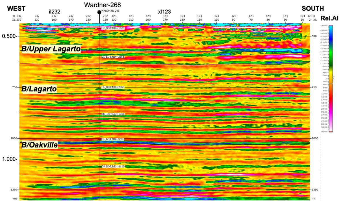
Figure 11. Typical line (combination of inline and crossline) showing results of inversion: (A) Acoustic impedance, showing the strong compaction trend and (B) relative acoustic impedance (RAI), with the compaction trend removed.
