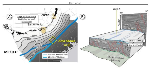
Figure 1. (A) Location map showing simplified structural contours on top of the Eagle Ford. Yellow box shows approximate location of dataset used in this study. (B) Annotated seismic imagery showing broad-scale structural configuration, ages of main stratigraphic units, and approximate location of the well used in this paper. This paper focuses on the Upper Cretaceous and Tertiary section above the Eagle Ford.
