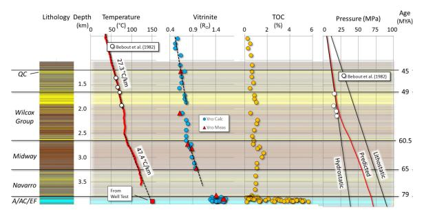
Figure 2. Left to right: Lithology profile derived from the gamma-ray log (yellow, sand; brown, shale; and blue, carbonates). Temperature profile (from measurement-while-drilling), vitrinite reflectance (measured and calculated from  $T_{max}$ ), predicted pore pressure, and calculated sedimentation rates. Stratigraphic names include the Queen City (QC) and Anacacho/Austin Chalk/Eagle Ford (A/AC/EF) interval at the base.
