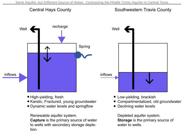
Figure 3. Schematic diagram and summary contrasting the Middle Trinity Aquifer in adjacent areas of Central Texas.
