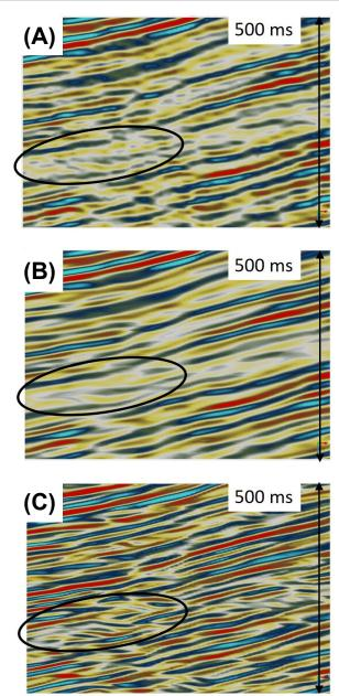
Figure 3. Cross-section on: (A) original seismic data, (B) original seismic data with structural filter, and (C) spectral extrapolation. Note that the spectral extrapolation sharpens the apparent downlapping features (black circles) and other stratigraphic details.
