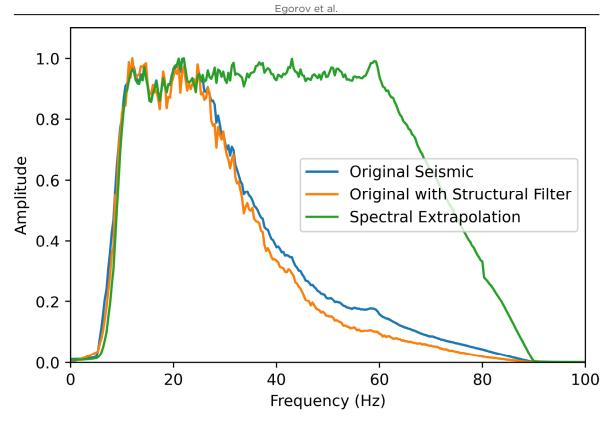
Figure 2. Spectra for the original seismic data (blue), structurally filtered original seismic data (orange), and spectral extrapolation (green). Note that high frequencies are preferentially canceled by the structural filter. The spectral extrapolation significantly widens the band.
