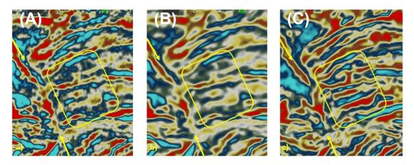
Figure 4. Time slices on: (A) original seismic data, (B) original seismic data with structural filter, and (C) spectral extrapolation. Note that the spectral extrapolation enhances more subtle details and improves continuity (in yellow outline). A large fault is also highlighted by the yellow arrows.
