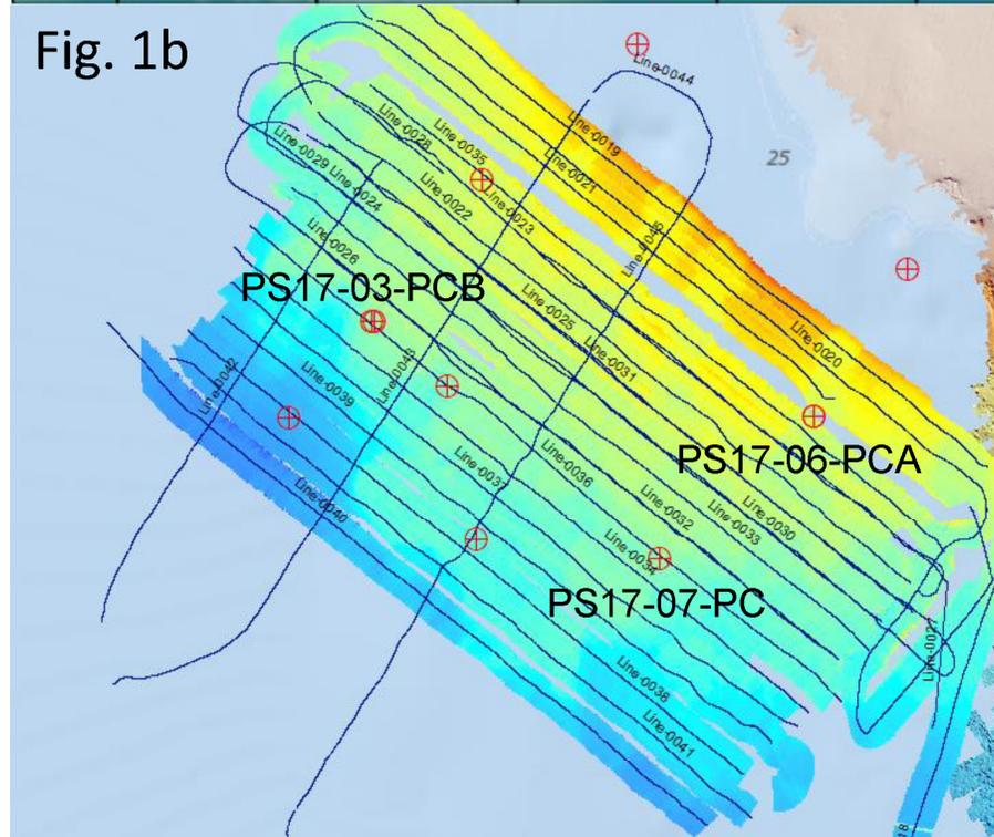
Figure 1. (a) Mississippi River Delta Front proximal to the subaerial structures of the Balize lobe “birdsfoot” (modified after Maloney et al., 2018). Study area highlighted in red. (b) Results of the 2016 Point Sur bathymetric survey of the Southwest Pass and selected cores.
