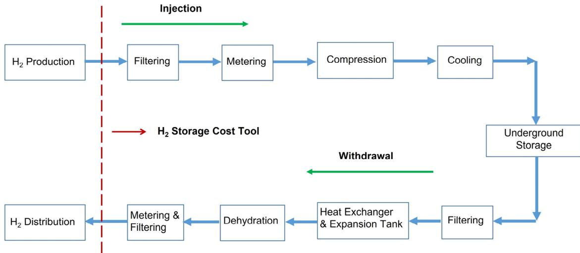
Figure 1. Hydrogen storage schematic.
