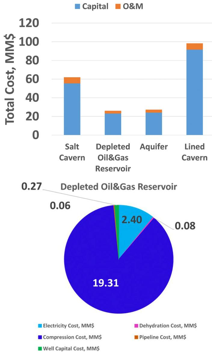
Figure 5. Capital and O&M cost by site type comparison (top) and depleted oil and gas reservoir costs (bottom). Aquifer costs (not shown here) are very similar to those costs for oil and gas reservoirs.
